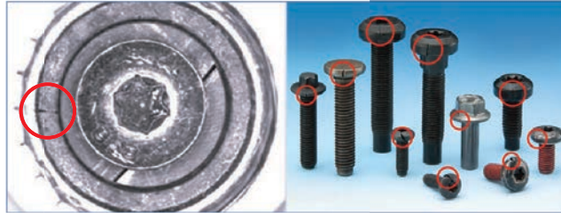
螺絲螺栓的輪裂檢測 Wheel crack of bolts
