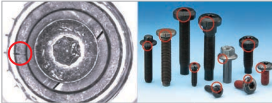
螺絲螺栓的輪裂 Wheel Crack of Bolts and Screw
