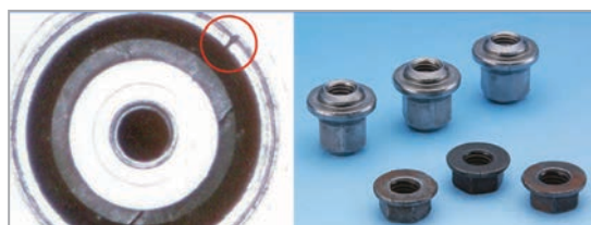
凸緣螺帽輪裂 Wheel crack of flange nut
