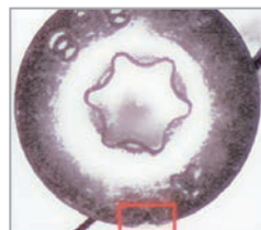
頭上裂痕 Head Crack
