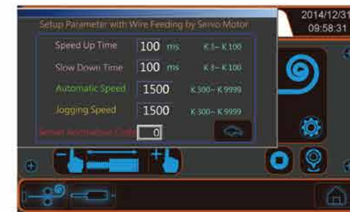
送料、擋料及後托系統的圖形操作面板 Wire Feeding, Stopper, K.O. Operated by Graphical Panel
