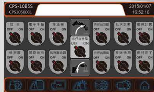
送料、擋料及後托系統的圖形操作面板 Wire Feeding, Stopper, K.O. Operated by Graphical Panel
