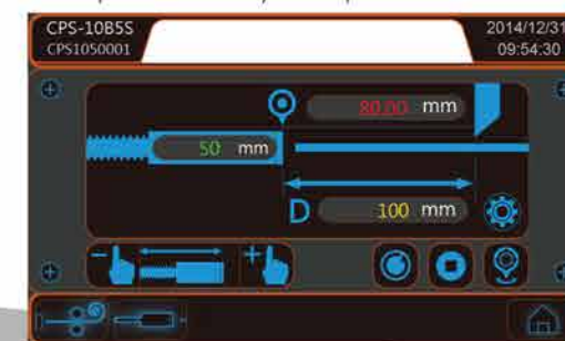
送料、擋料及後托系統的圖形操作面板 Wire Feeding, Stopper, K.O. Operated by Graphical Panel
