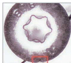
頭上裂痕 Head Crack
